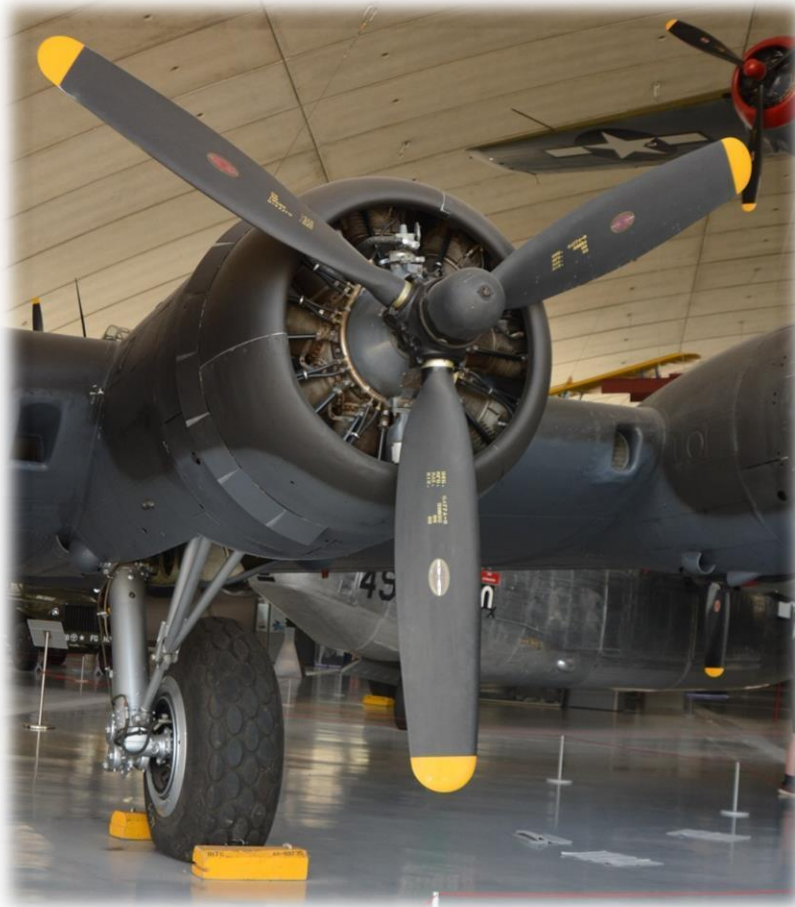
Wright R-1820-97 "Cyclone" turbo supercharged radial engine, 1,200 hp
